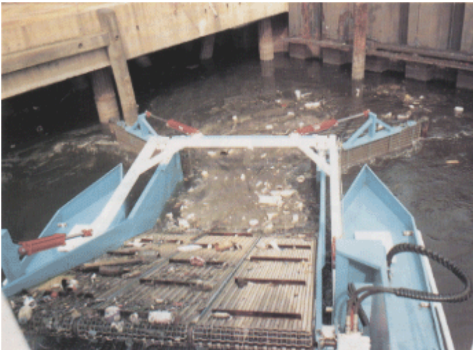
Figure 5-16 TrashCat’s conveyORIZED wings let it collect debris in tight corners Source: http://www.trashskimmer.com/
